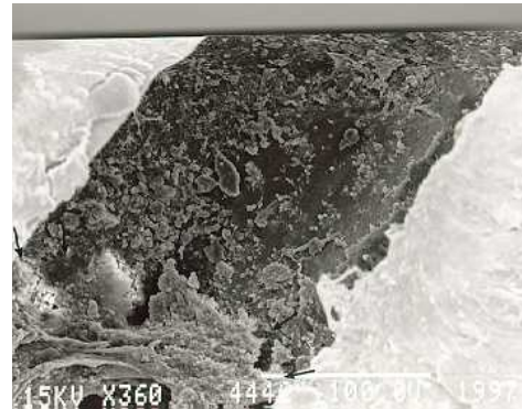
Image 5: On top, clean surface of channel. Down, the area not reached by probe
